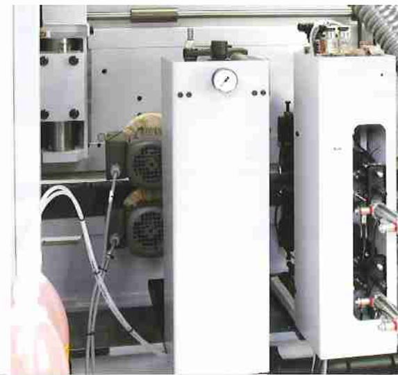
Finish processing FA 10 Comprising a glue joint scraping device for disposal of glue residues above and below on PVC edges.
