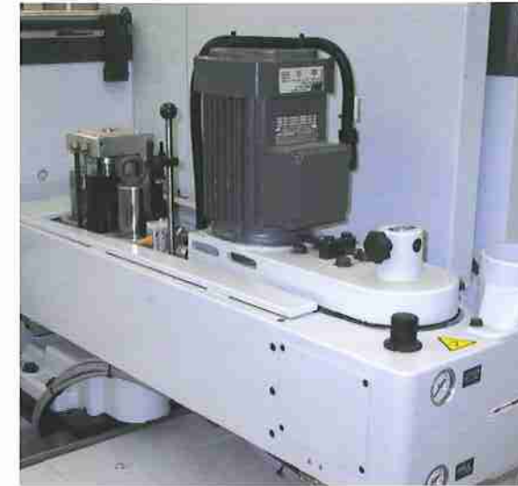
Belt sanding unit KS 10 For sanding straight veneer and solid edges.
