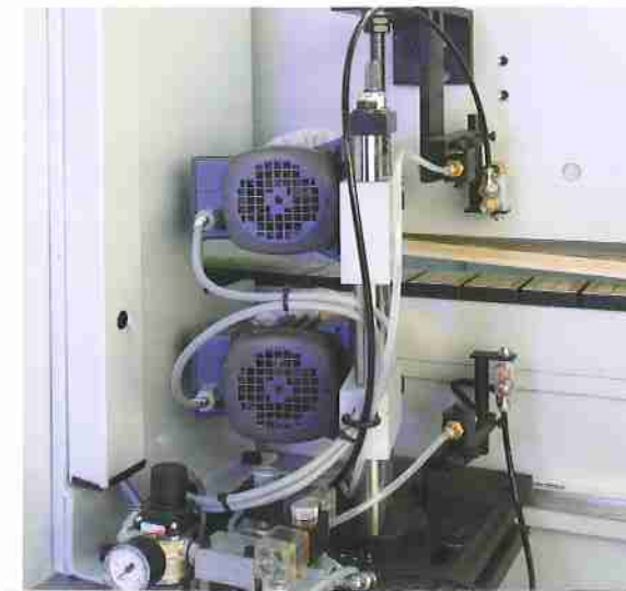
Buffing unit above and below with oscillation To smooth off edges utilizing the entire disk width.
