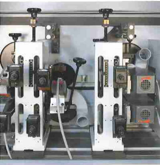
Rough trimming unit For rough trimming the upper and lower edge overhang.
