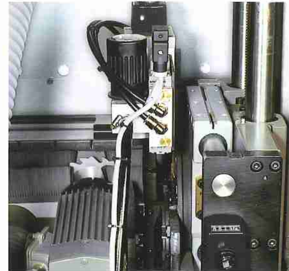
Universal trimming unit UF 11 For grooving, rebating and profiling with swivel-action and controlled motor.
